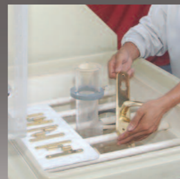
The protective surface layer of each handle has been checked for its resistance to corrosion.
