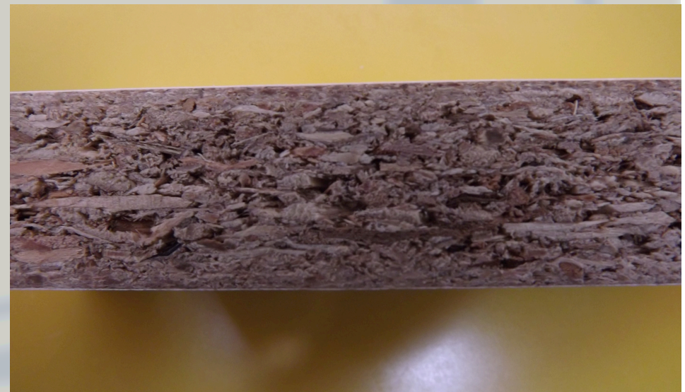
MFC with riven core retains water and bacteria
