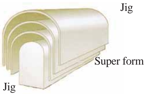
Fig : (a) Jig method for multiple shapes
