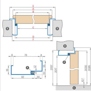
1) allowable deviation due to frame dimensional tolerance of +- 3mm (we recommend to check before installation)
