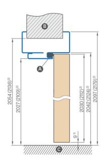
$<sup>^{1)}</sup>$  allowable deviation due to frame dimensional tolerance of +- 3 mm (we recommend to check before installation)
