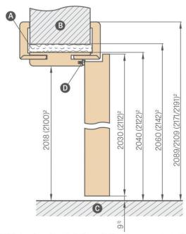
$<sup>^{1)}</sup>$  allowable deviation due to frame dimensional tolerance of +- 3 mm (we recommend to check before installation)
