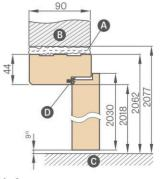
1) allowable deviation due to frame dimensional tolerance of +- 3 mm (we recommend to check before installation)
