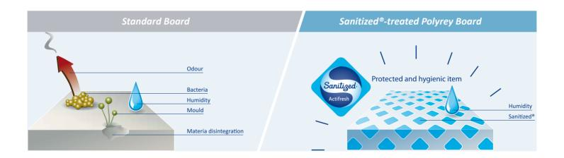
Integrated within the material in order to assure antibacterial protection throughout its lifecycle, this biocidal additive does not influence the technical and aesthetic performances of our HPL and Compact products.
